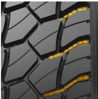
Stone Protectors to extend casing life
