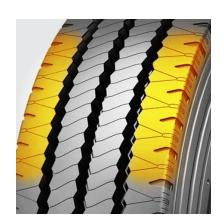
Siping for added traction in wet and icy conditions
