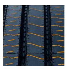
Stone ejectors protect tire from stone drilling.
