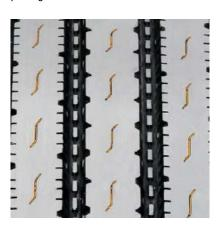
Stone ejectors protect tire from stone drilling.
