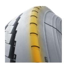
Stone ejectors protect tire against stone drilling.
