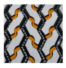
Stone ejectors protect tire against stone drilling.
