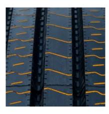
Stone ejectors protect tire from stone drilling.
