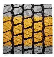
Extensive sipes improve traction in wet conditions and dissipate heat for prolonged tread life.
