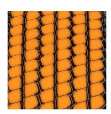
Zig-zag circumferential grooves provide additional biting edges for increased traction.
