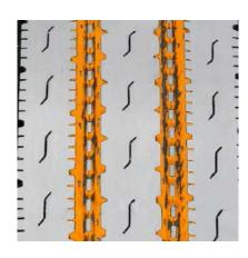
Decoupling groove helps to minimize irregular wear.
