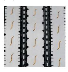
Stone ejectors protect tire from stone drilling.
