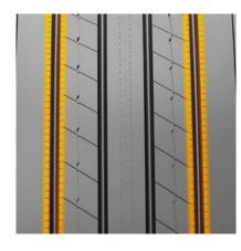
Shallow five-rib design and Advanced Compound Technology for low rolling resistance
