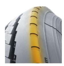
Stone ejectors protect tire against stone drilling.
