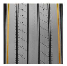
Micro-sipes improve traction in wet conditions and dissipate heat for prolonged tread life
