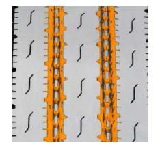
Decoupling groove helps to minimize irregular wear.
