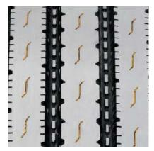
Stone ejectors protect tire from stone drilling.
