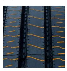
Stone ejectors protect tire from stone drilling.
