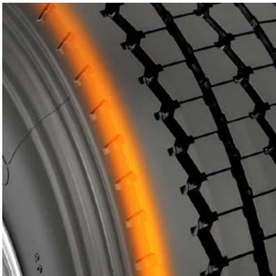
Engineered tread design provides low rolling resistance and improved efficiency.
