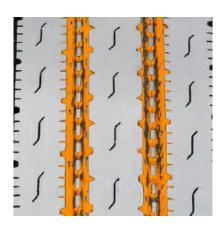
Decoupling groove helps to minimize irregular wear.
