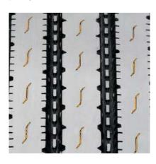
Stone ejectors protect tire from stone drilling.
