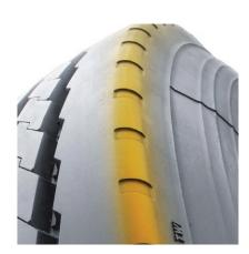
Stone ejectors protect tire against stone drilling.
