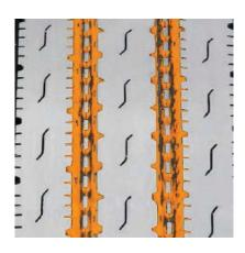
Decoupling groove helps to minimize irregular wear.
