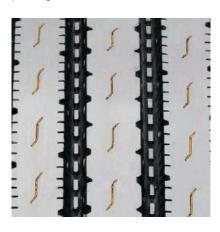
Stone ejectors protect tire from stone drilling.
