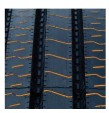
Stone ejectors protect tire from stone drilling.
