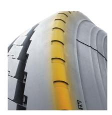
Stone ejectors protect tire against stone drilling.
