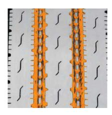
Decoupling groove helps to minimize irregular wear.
