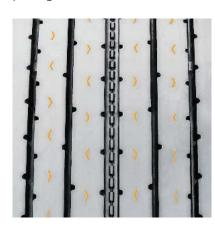
Main groove stone ejectors protect tire against stone drilling
