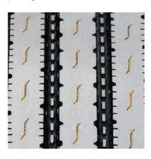
Stone ejectors protect tire from stone drilling.
