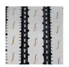
The S605 EFT is Sailun's premium line-haul steer tire, featuring a decoupling groove and five wide ribs for a stable ride at all speeds. Stone ejectors minimize tire damage, while extra-wide grooves and S-sipes improve traction for excellent hydroplaning resistance.
