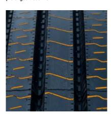
Stone ejectors protect tire from stone drilling.
