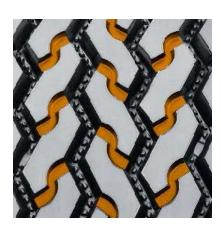
Stone ejectors protect tire against stone drilling.
