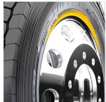
“Slim bead” for reduced rolling resistance.
