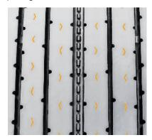
Main groove stone ejectors protect tire against stone drilling
